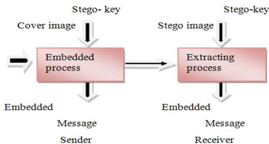
Figure 1: General Block Diagram of Steganography
